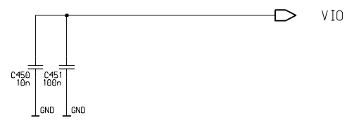
Decoupling capacitors for 1st flash
